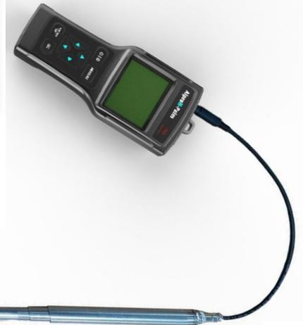
DIRECT MEASUREMENT OF DISSOLVED HYDROGEN IN ALUMINUM ALLOYS
